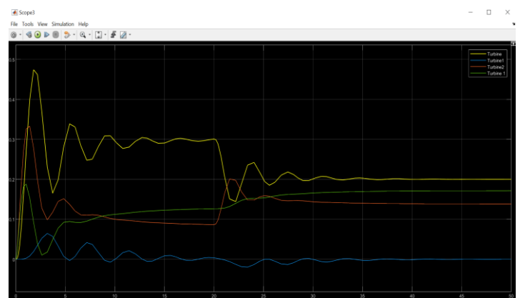
Fig 11: The results of the turbines in the MIMO process after application of PID and Fuzzy control.
