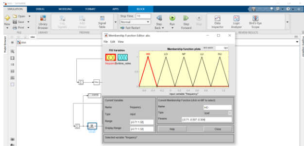
Fig 7: Input membership functions for the Fuzzy rules applied to both SISO and MIMO
