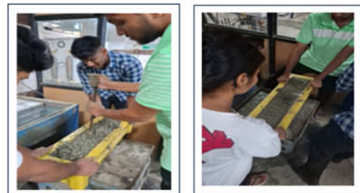
Fig.4.3 Casting of Concrete
