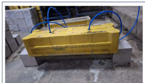
Fig.4.3 Curing using air compressor
