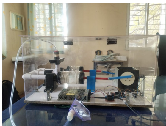
Fig.9 The Project displaying Oxygen purifying process using bellows and slider crank mechanism to the breathing channel using mask.
