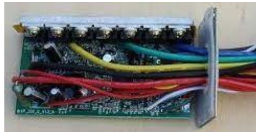
Fig-4: BLDC Motor Controller for Hybrid E-Bicycle
